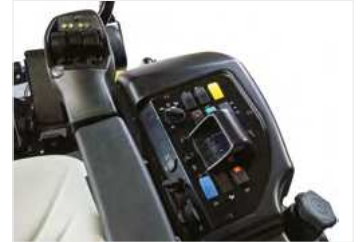
Operator lift lower controls & onboard diagnostics
