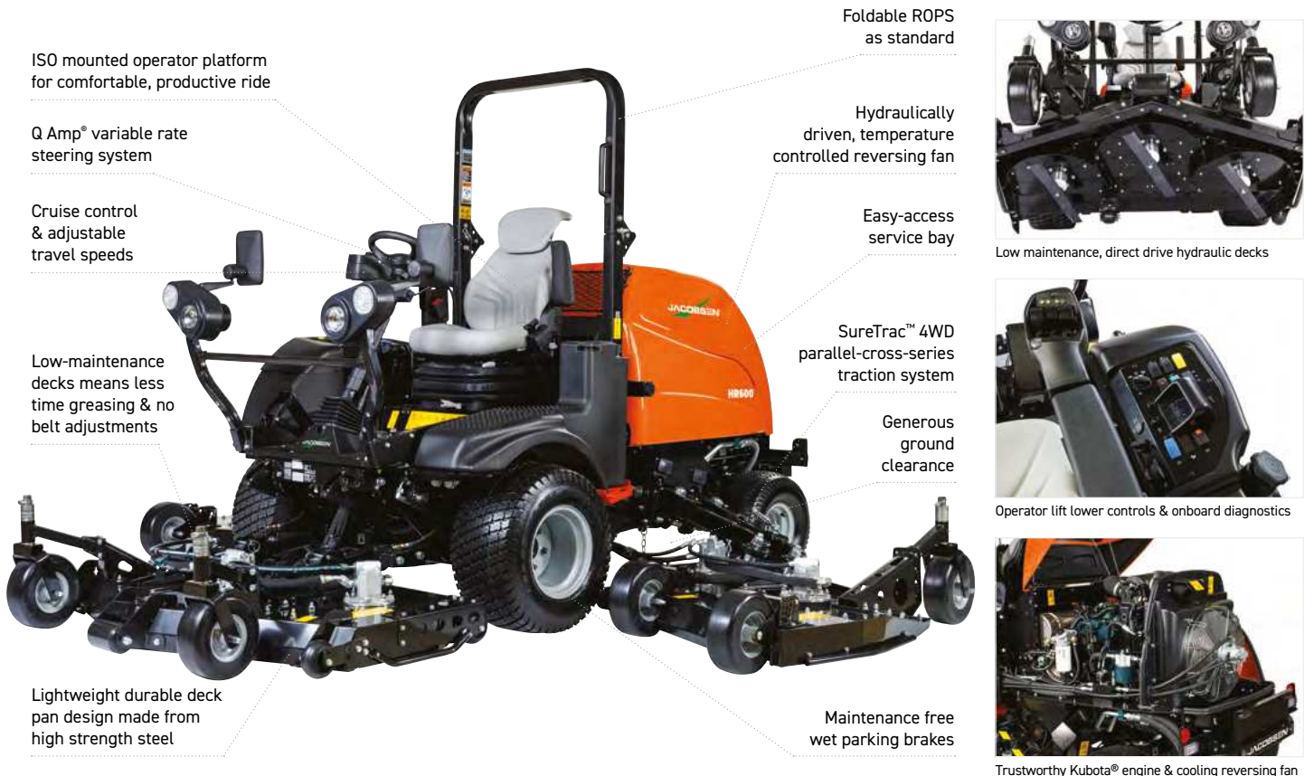
Trustworthy Kubota® engine & cooling reversing fan
