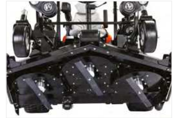
Low maintenance, direct drive hydraulic decks
